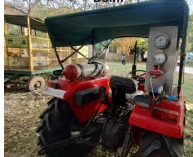
CBG-Biodiesel powered Dual-fuel Tractor, CRDT, IIT Delhi
