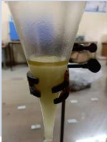
Step-5 Separation of biodiesel layer from glycerol
