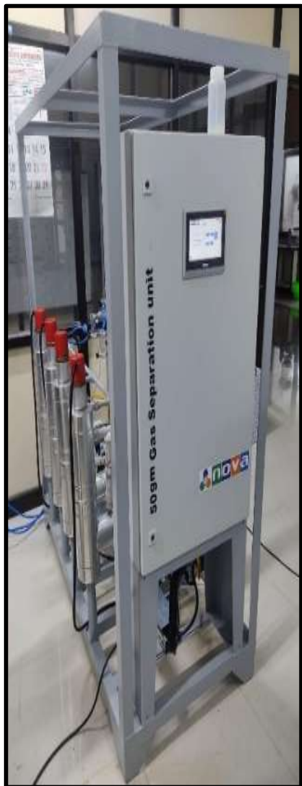
Fabricated gas adsorption units (50g, 1 kg, 25 kg)
