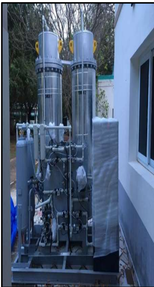
Fabricated gas adsorption units (50g, 1 kg, 25 kg)
