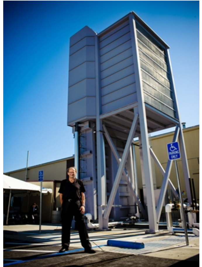
CTO and co-founder Peter Eisenberger in front of Global Thermostat's air-capturing machine.
