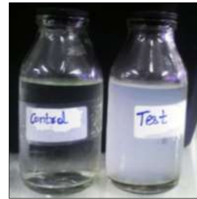
Analysis of carbonate precipitation catalyzed by crude and pure preparations of BhCA. BSA served as a negative control. Specific inhibition of purified BhCA by AZA led to decline in carbonate precipitation
