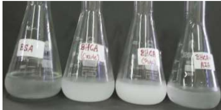
Analysis of carbonate precipitation catalyzed by crude and pure preparations of BhCA. BSA served as a negative control. Specific inhibition of purified BhCA by AZA led to decline in carbonate precipitation
