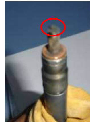
Heavily Scored Injector Pintle with Untreated Fuel
