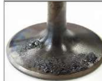
Heavily Scored Inlet Valve with Untreated Fuel
