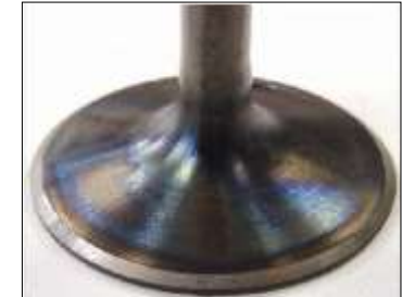
Clean Inlet Valve with additive treated Fuel
