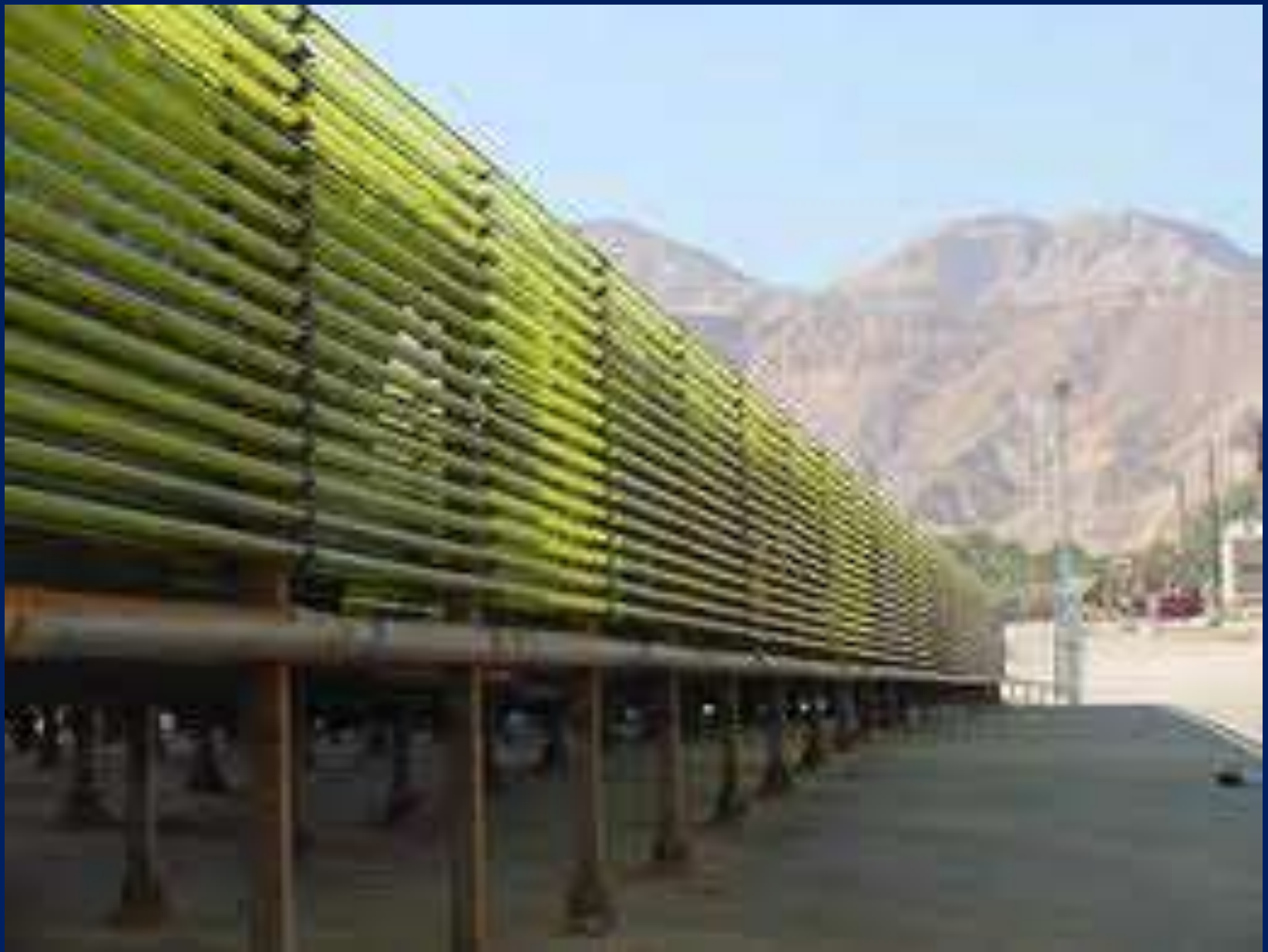
Algal cultivation in horizontal Glass tubular column
