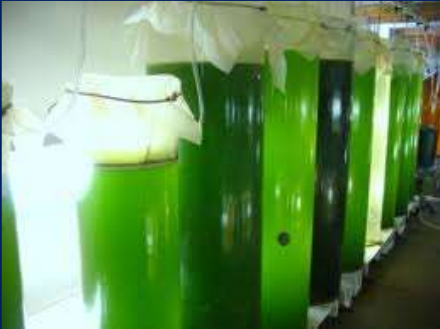
Algal cultivation using CO 2 in vertical Glass Containers
