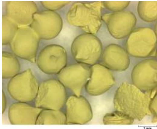
Pictures of UiO-Ni and CPO-27-Ni made by extrusion method.
