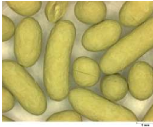
Pictures of UiO-Ni and CPO-27-Ni made by extrusion method.
