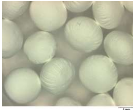
Pictures of UiO-Ni and CPO-27-Ni made by extrusion method.
